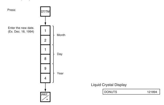
**NOTE:** The scale will check the details of the date input. An invalid date will result in an error.
